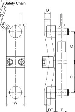
In many industrial applications the tension in wire rope needs to be carefully and continuously monitored.
