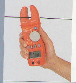
MS2600 IS AN OPEN JAW DIGIT ELECTRICAL TESTER. THERE ARE DCV. ACV, ACA, Ω, CAP, FREQUENCY, DIODE TEST, CONTINUITY TEST AND DUTY CYCLE TEST FUNCTION. OTHERWISE THERE ARE AUTO AND MANUAL RANGE, RELATIVE MEASUREMENT, DATA HOLD, AND BACKLIGHT AUTO OFF TIME LIMIT MODE.TEST LEADS CAN BE INSERTED ON GROOVE OF BACK OF THE TESTER.
