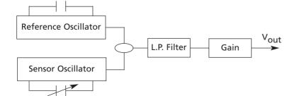
$V_{out} = V_{cc} * (0.00474 * \% RH + 0.2354)$
